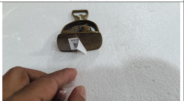
Tape test view
