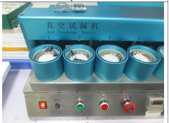
Waterproof test view
