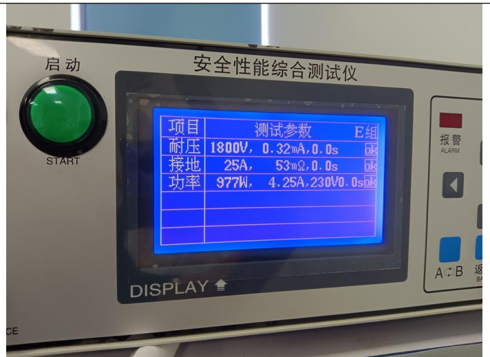
High voltage, grounding test
