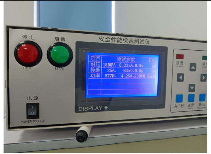
High voltage, grounding test
