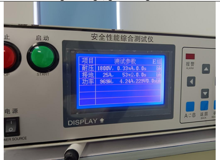
High voltage, grounding test
