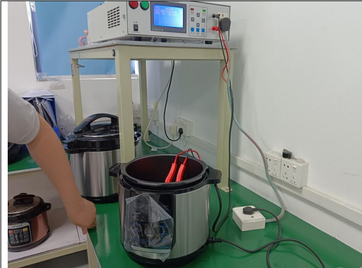
High voltage, grounding test
