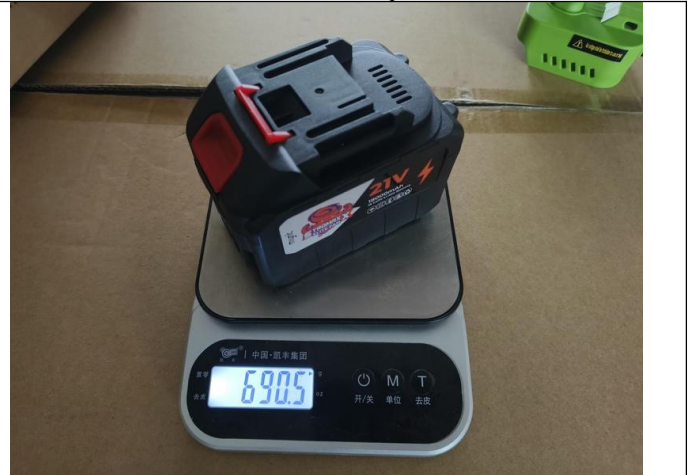
Battery weight check:690.5g
