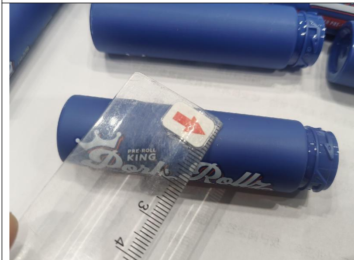
Paint stain on tube - Min
