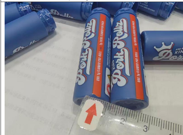
Poor printing on red line - Min
