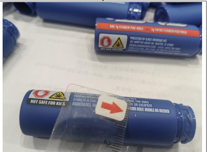
Paint stain on tube - Min
