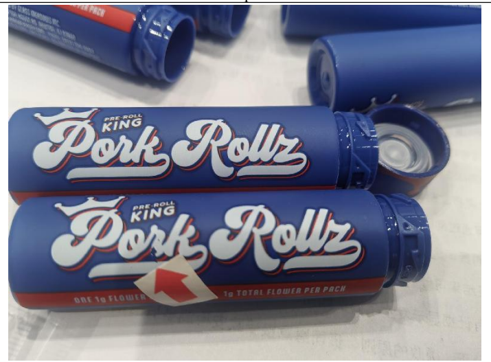
Poor printing on tube - Maj
