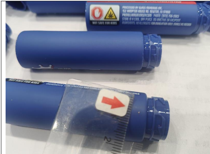
Paint stain on tube - Min
