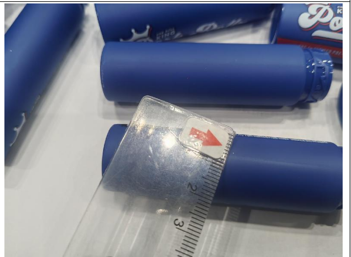
Paint stain on tube - Min
