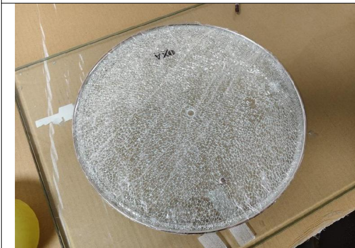
Inspection of tempered glass
