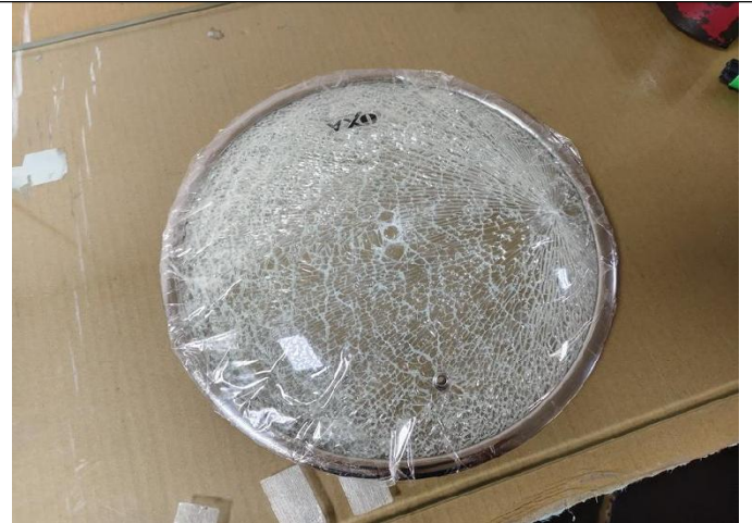
Inspection of tempered glass
