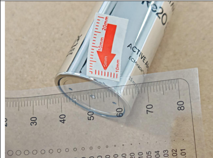
Dent mark on unit-Minor
