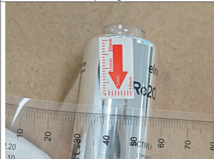
Scratch mark on unit-Minor
