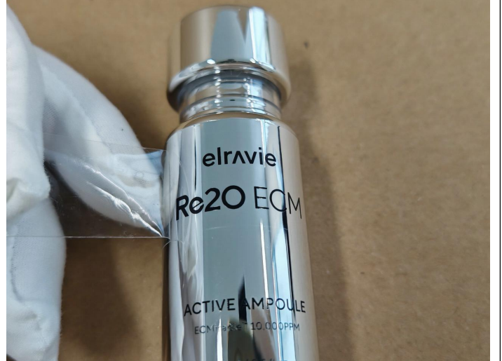
Silk Screen Printing Adhesive Test
