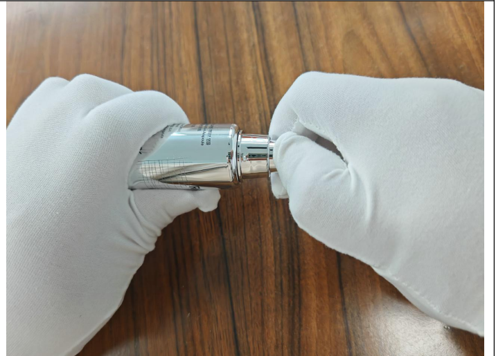
Pull test on Snaps
