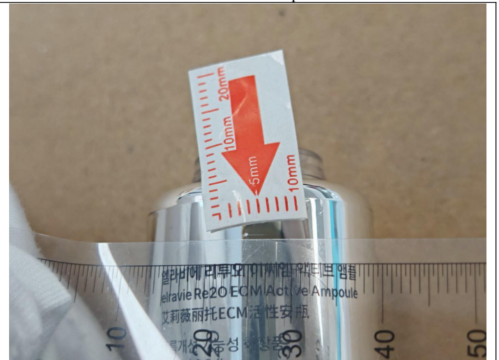
Scratch mark on unit-Minor
