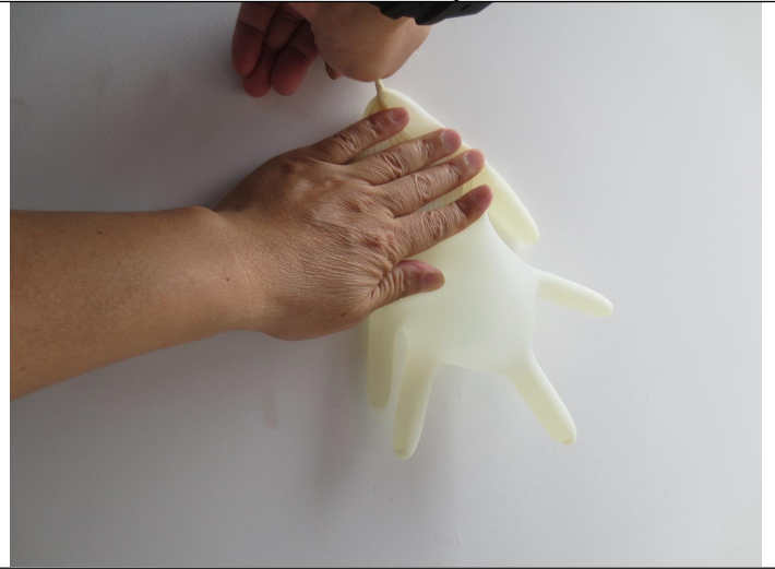
Leakage test view
