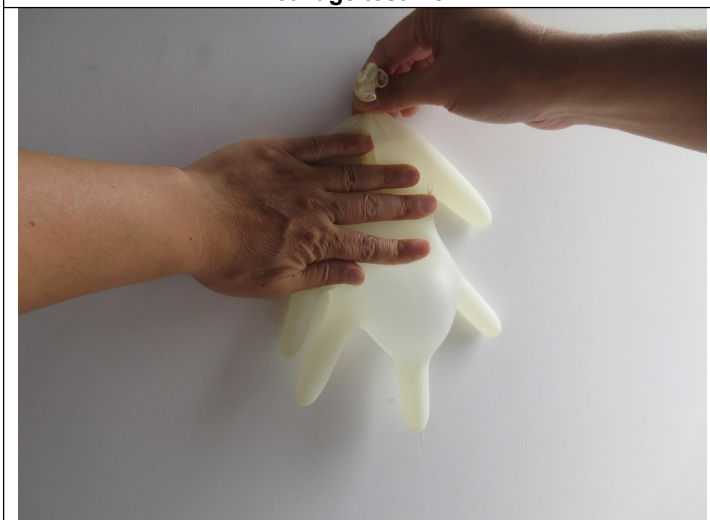
Leakage test view
