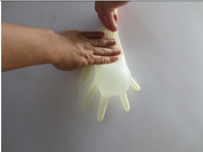
Leakage test view
