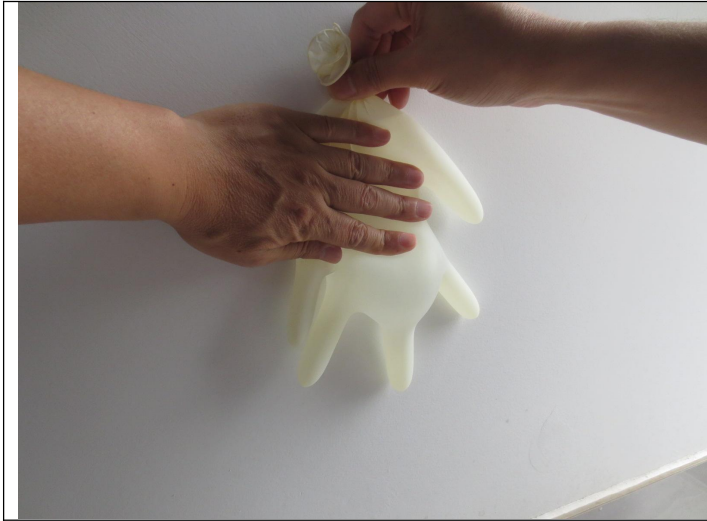
Leakage test view
