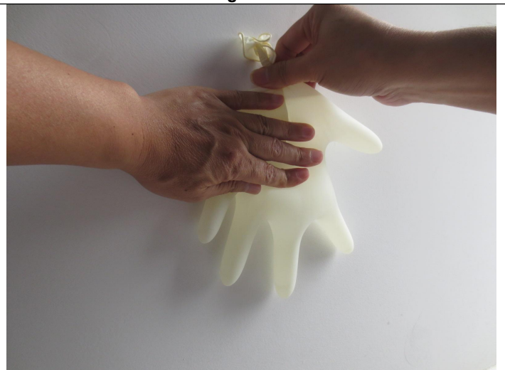
Leakage test view
