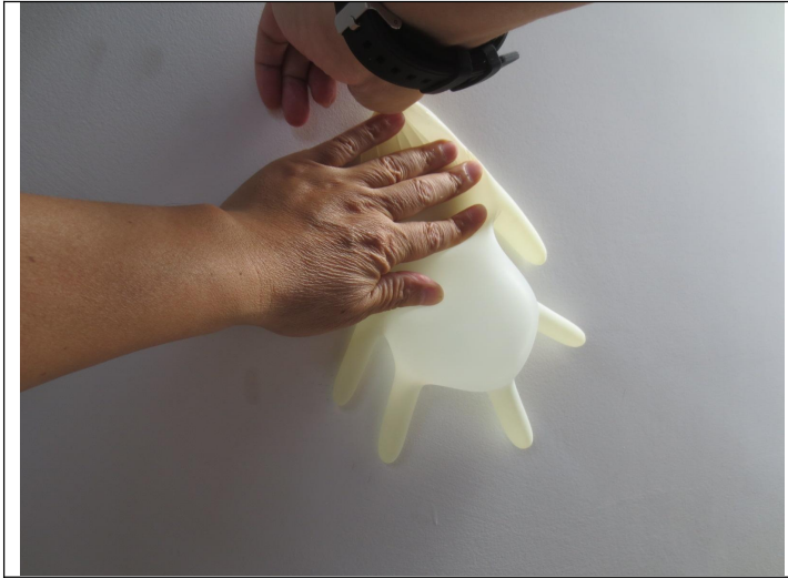
Leakage test view
