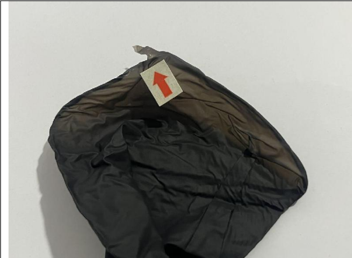
Poor edge curling -major
