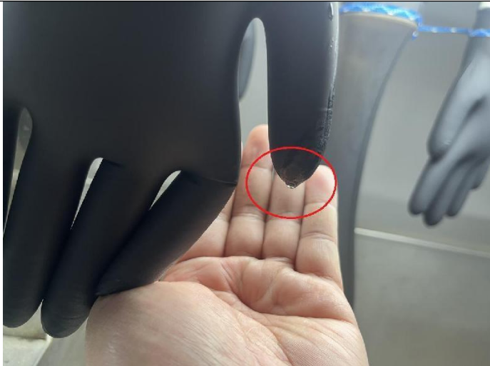
9. Thickness of the wrist and palm of the product is the same, while the thickness of the fingertip is a bit higher (the fingertip is rough).
