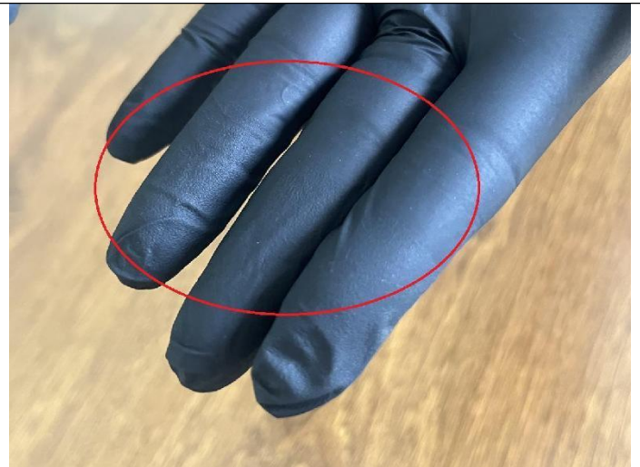
9. Thickness of the wrist and palm of the product is the same, while the thickness of the fingertip is a bit higher (the fingertip is rough).
