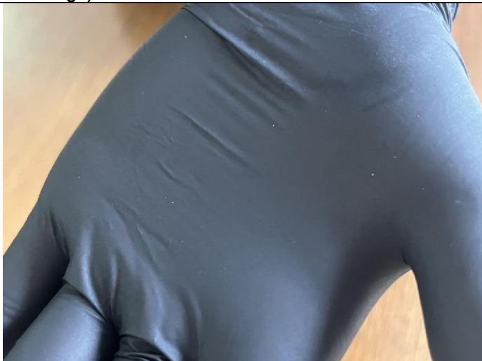
9. Thickness of the wrist and palm of the product is the same, while the thickness of the fingertip is a bit higher (the fingertip is rough).
