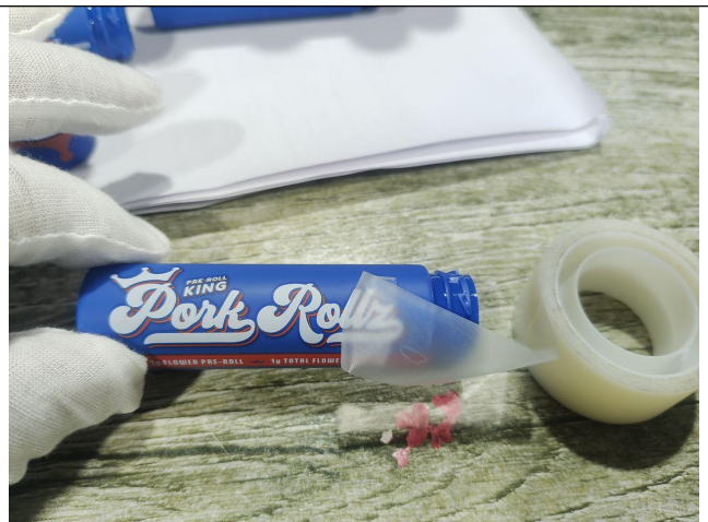
Silk Screen Printing Adhesive Test
