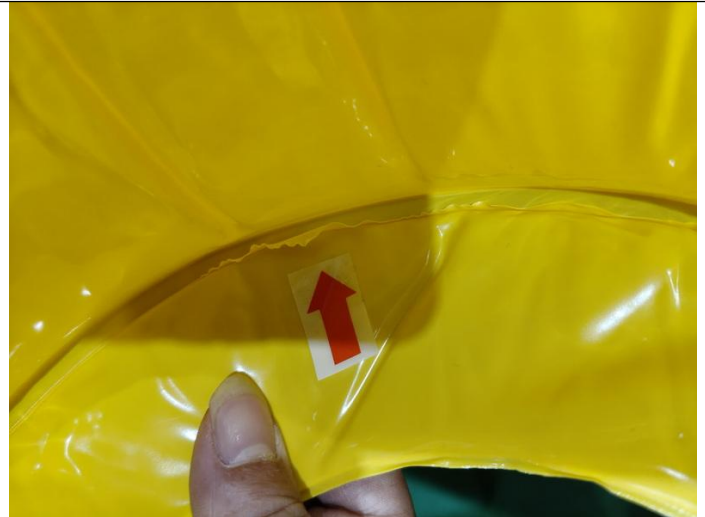
Poor cutting edge-Major
