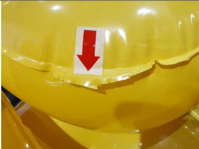
Poor cutting edge-Major
