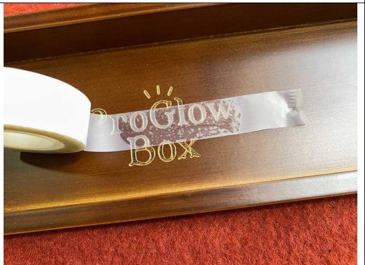
3M adhesive test
