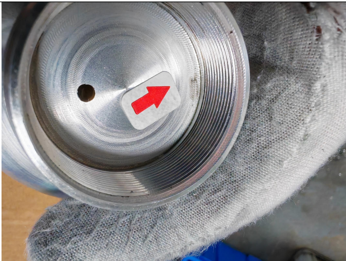
Oil stain on surface-Minor
