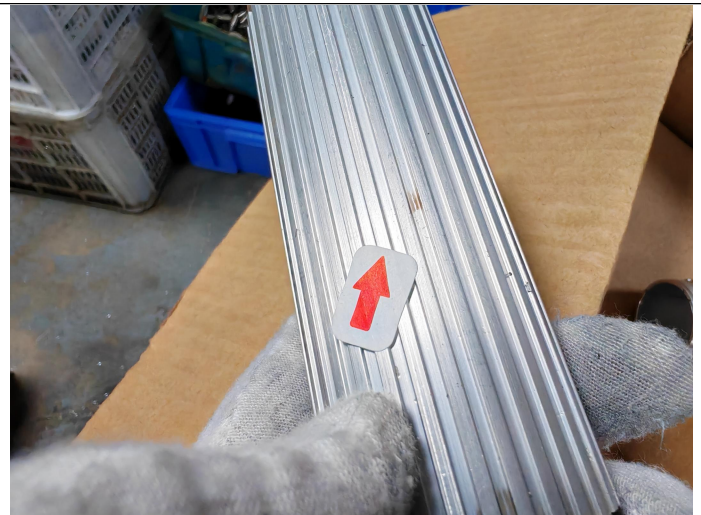
Oil stain on surface-Minor
