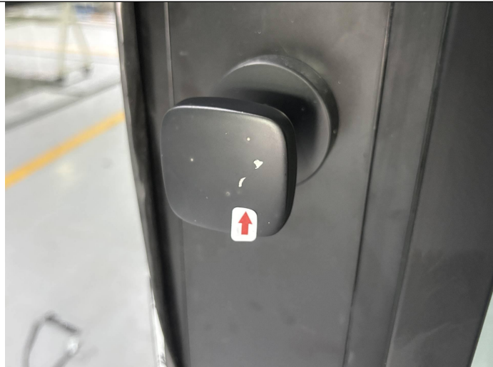
Scratch mark on unit-Major
