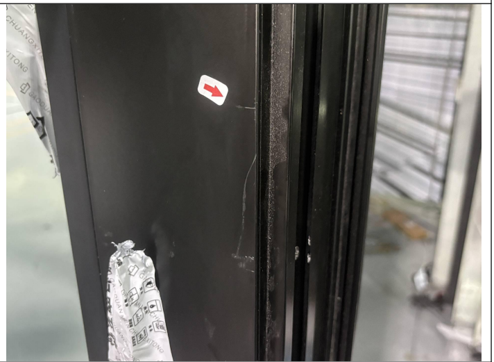
Scratch mark on unit-Major
