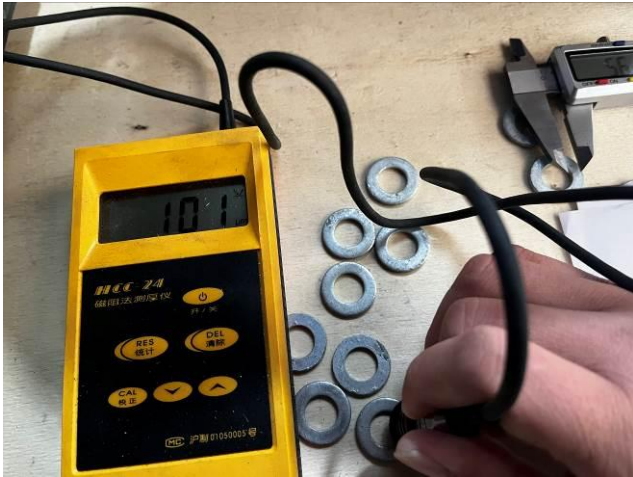
Zinc layer thickness test
