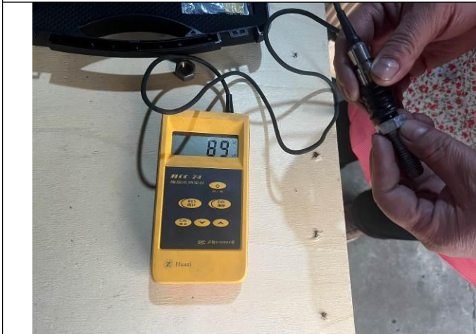
Zinc layer thickness test
