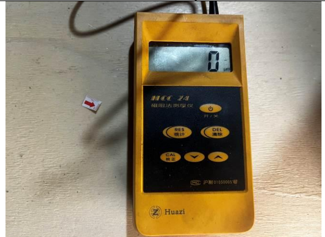
Zinc layer thickness test
