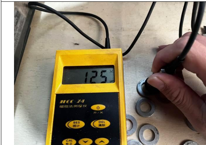
Zinc layer thickness test
