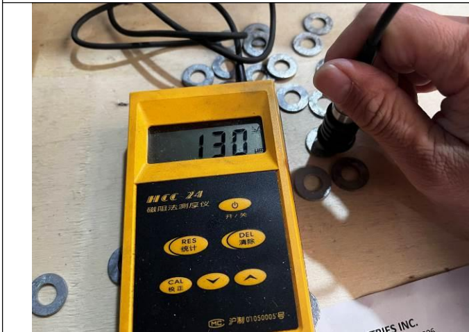
Zinc layer thickness test
