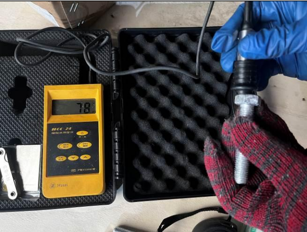
Zinc layer thickness test
