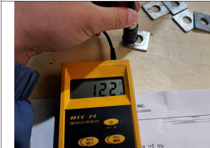
Zinc layer thickness test
