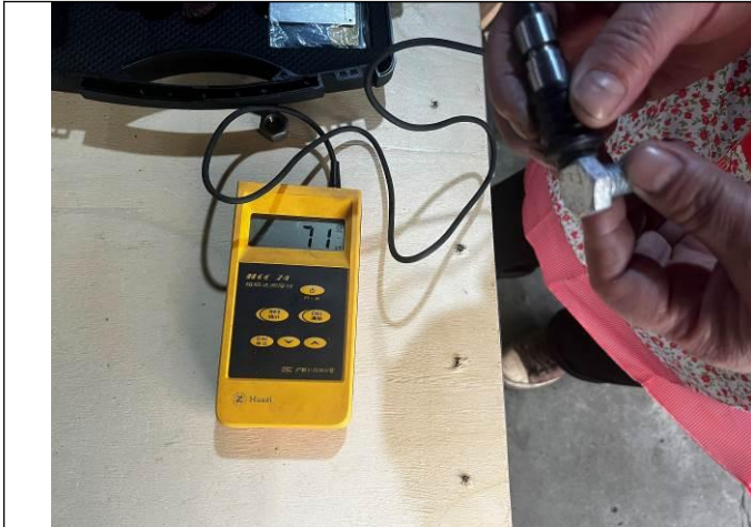
Zinc layer thickness test
