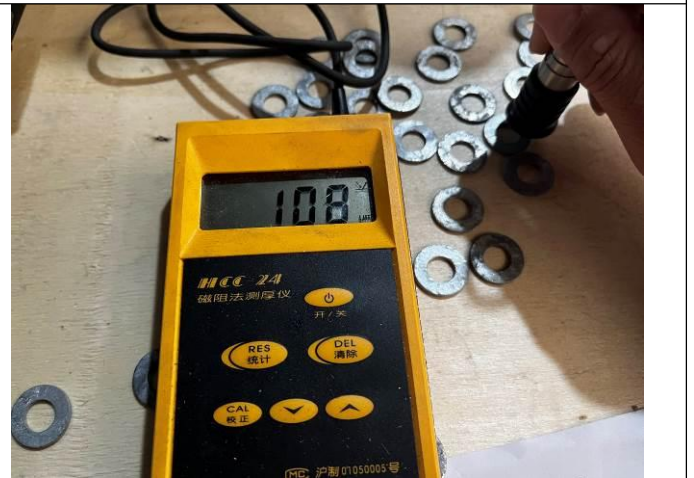
Zinc layer thickness test
