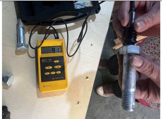
Zinc layer thickness test
