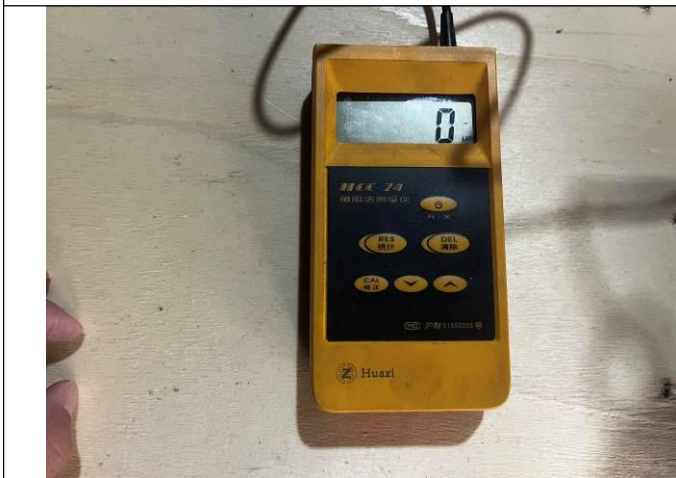
Zinc layer thickness test
