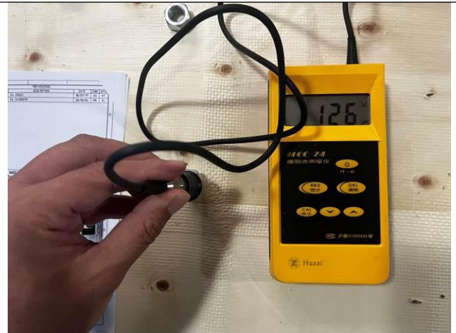
Zinc layer thickness test
