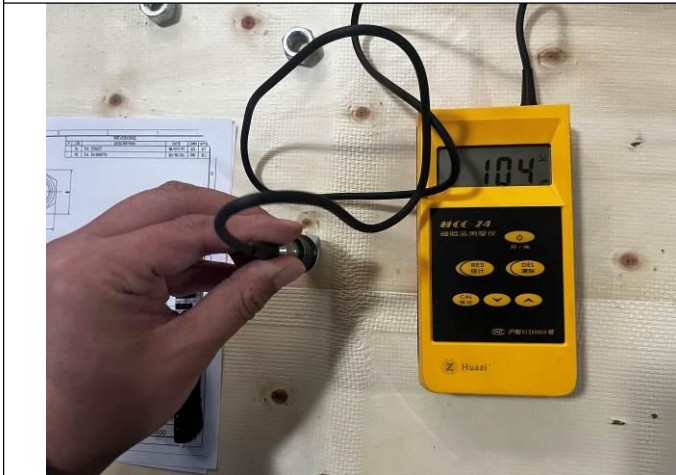
Zinc layer thickness test
