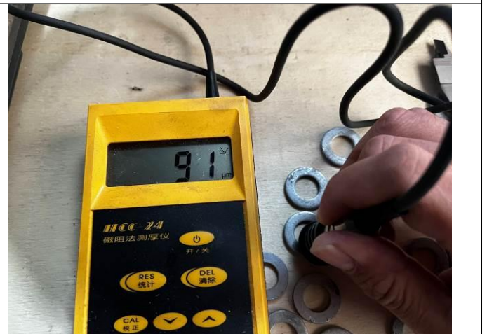
Zinc layer thickness test
