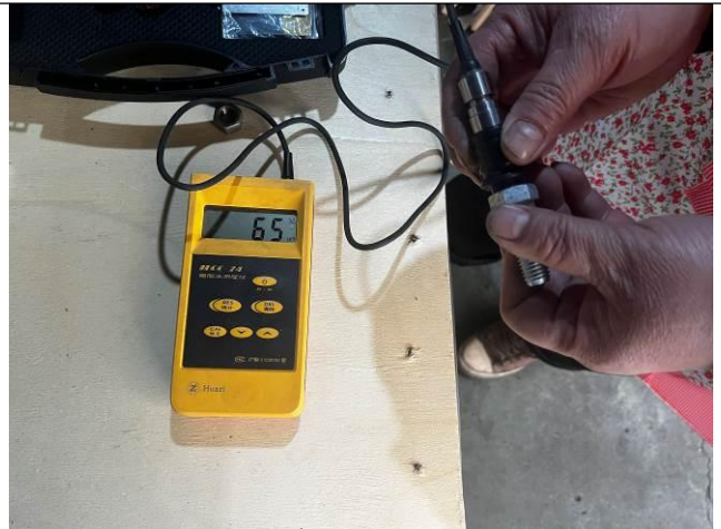
Zinc layer thickness test
