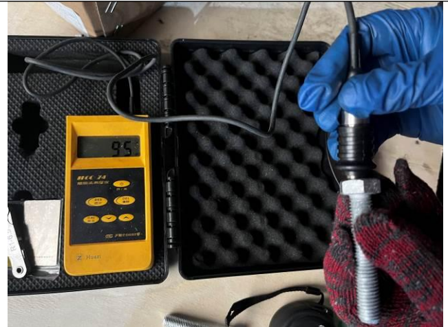
Zinc layer thickness test
