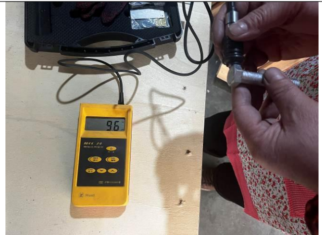
Zinc layer thickness test
