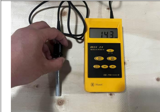
Zinc layer thickness test
