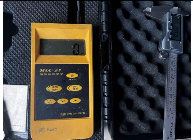
Zinc layer thickness test
