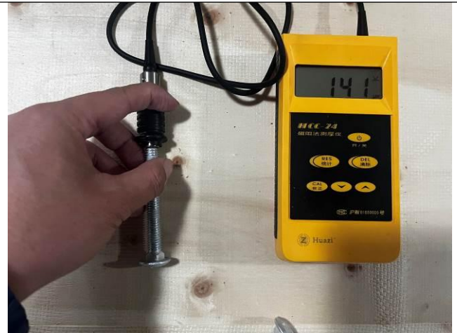
Zinc layer thickness test
