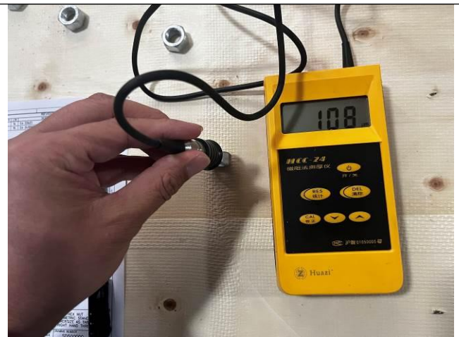
Zinc layer thickness test
