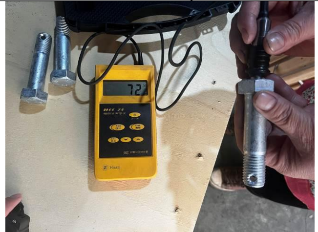
Zinc layer thickness test
