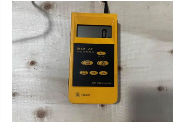
Zinc layer thickness test
