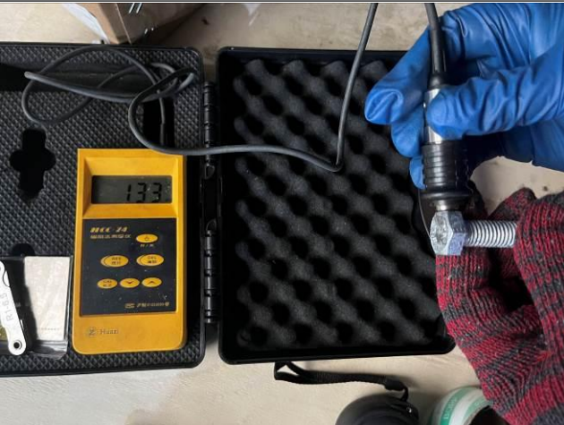
Zinc layer thickness test
