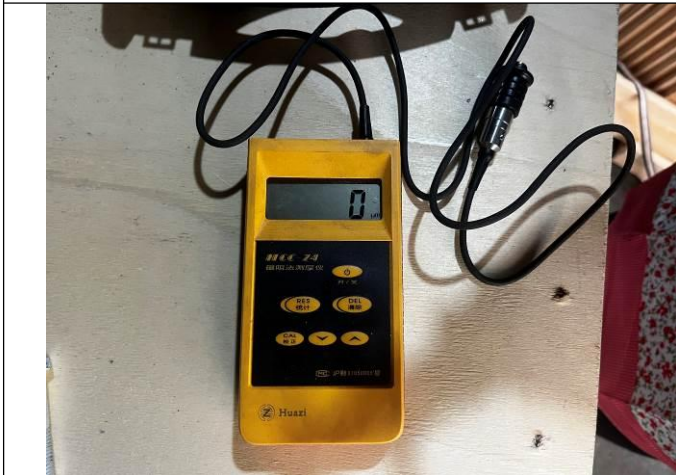
Zinc layer thickness test
