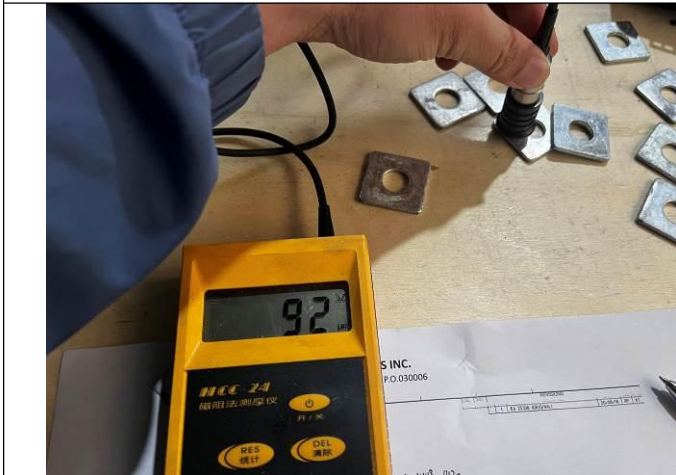
Zinc layer thickness test
