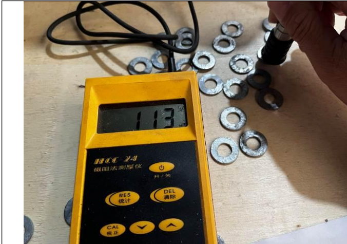
Zinc layer thickness test
