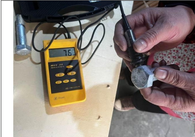
Zinc layer thickness test
