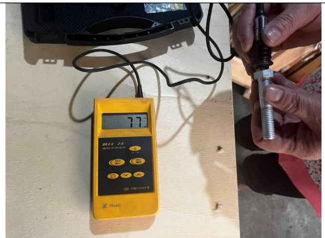
Zinc layer thickness test
