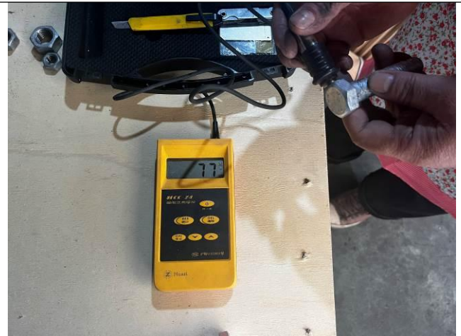
Zinc layer thickness test
