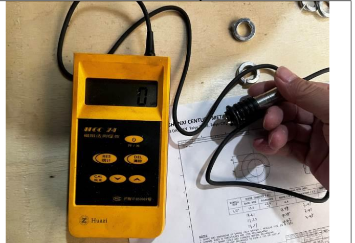
Zinc layer thickness test
