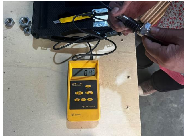
Zinc layer thickness test
