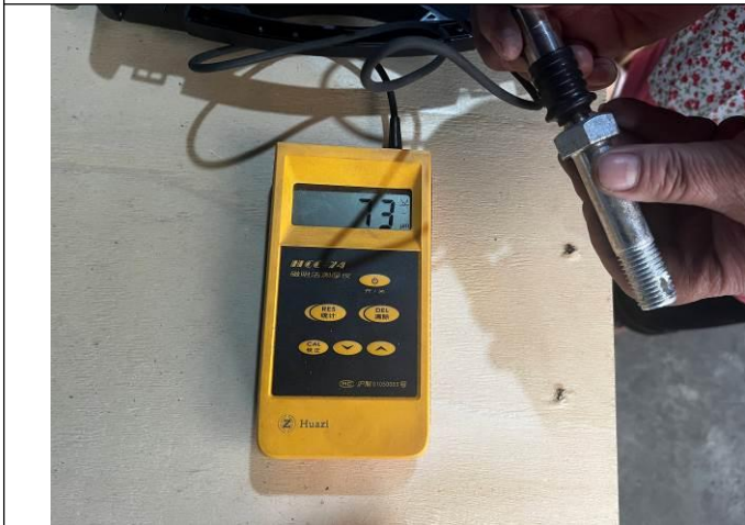
Zinc layer thickness test
