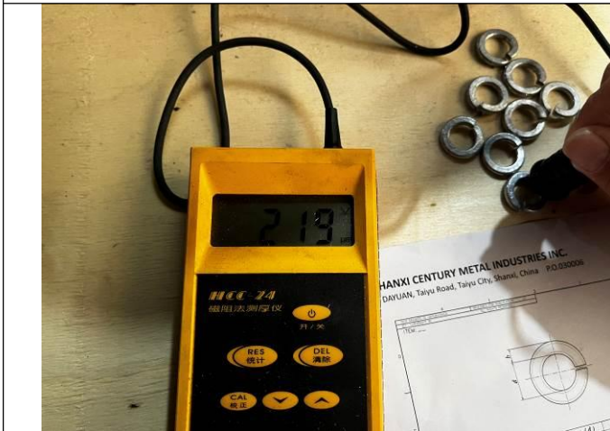
Zinc layer thickness test
