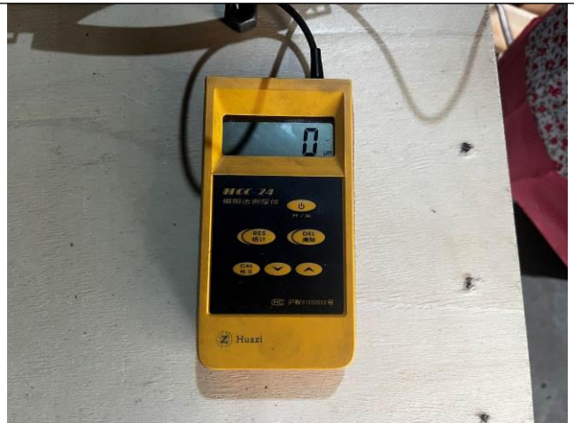
Zinc layer thickness test
