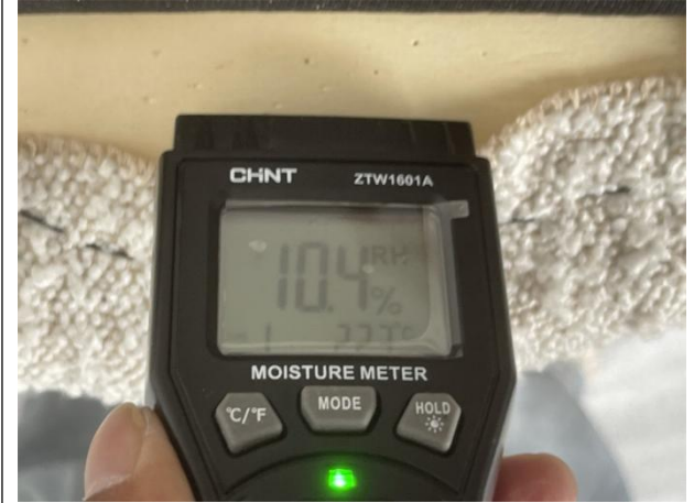
Humidity test-Testing the humidity of the wooden structure-S2
