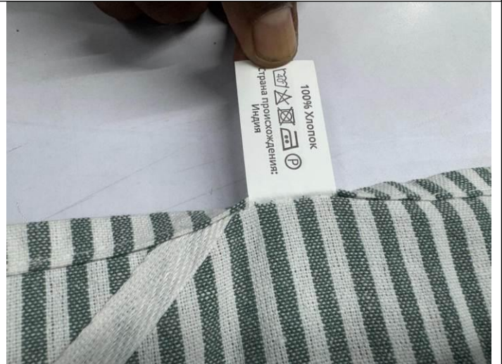
LABEL PULLING TEST
