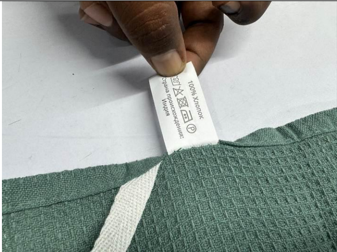
LABEL PULLING TEST
