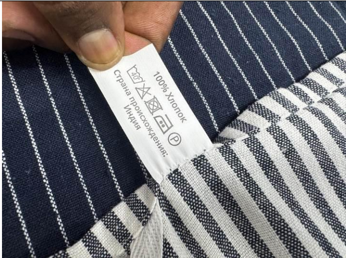
LABEL PULLING TEST
