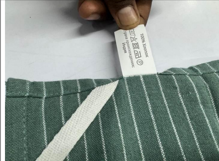
LABEL PULLING TEST
