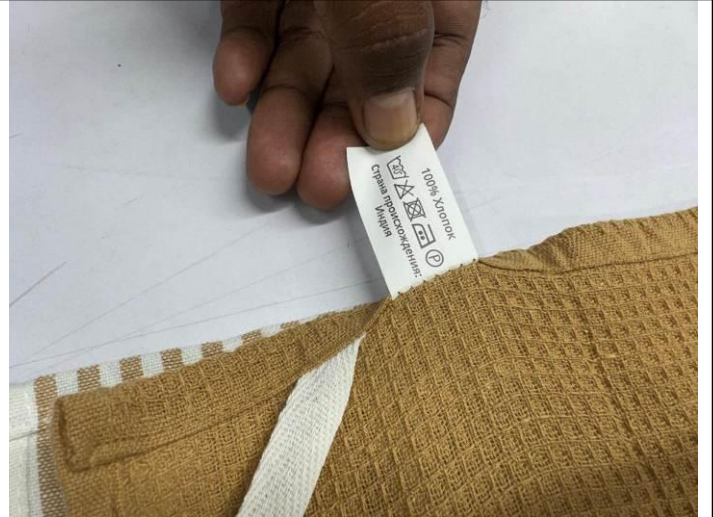
LABEL PULLING TEST
