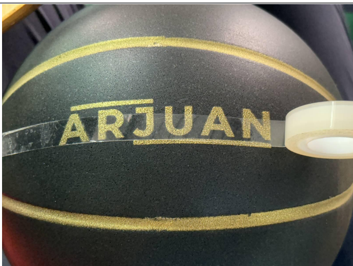
Silk Screen Printing Adhesive Test
