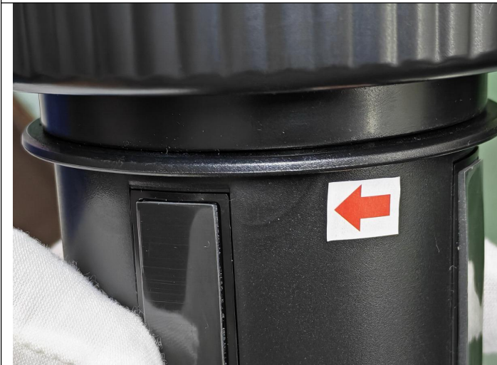
Water wave mark on surface-minor
