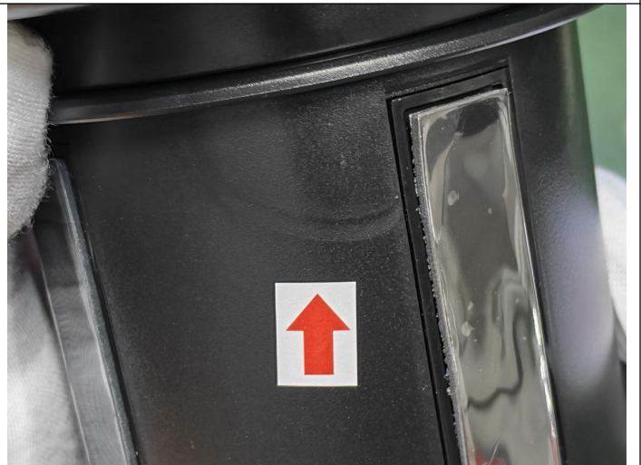
Water wave mark on surface-minor
