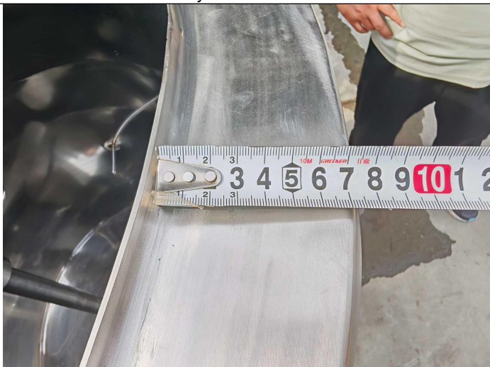
The insulation layer thickness is approximately 70 mm.
