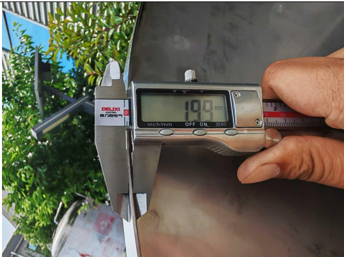
The outer layer thickness is 1.99 mm.
