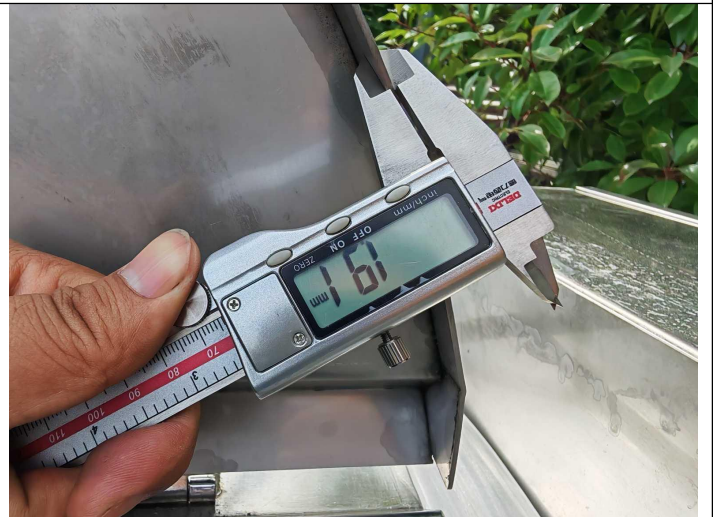
The outer layer thickness is 1.91 mm.
