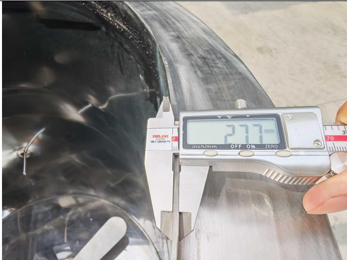
The inner tank wall thickness is 2.77 mm.
