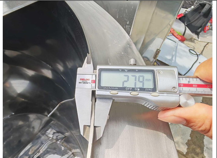
The inner tank wall thickness is 2.79mm.
