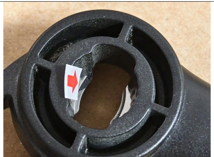
Excessive flash -Minor
