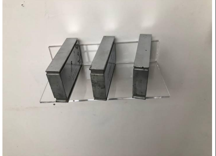
Static loading test
