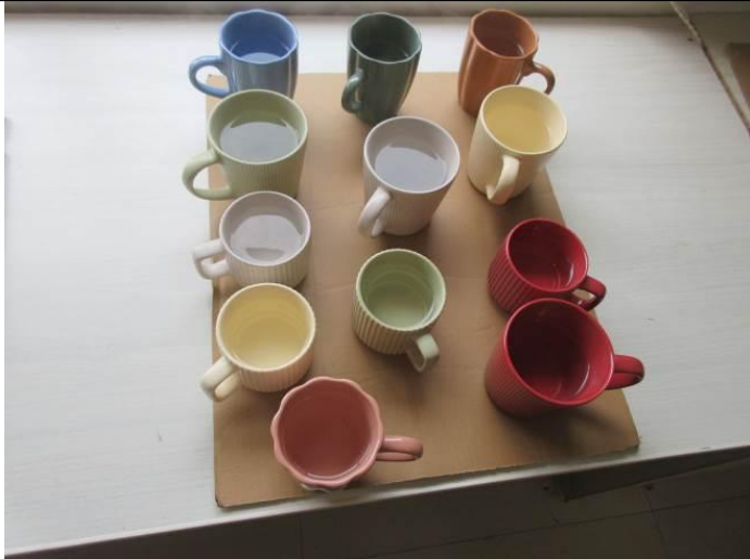
Boiling water test / Leakage test
