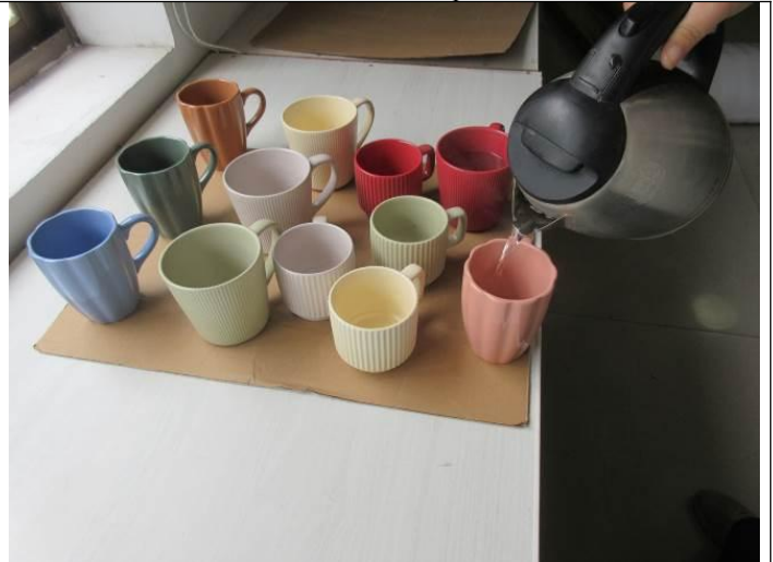
Boiling water test / Leakage test
