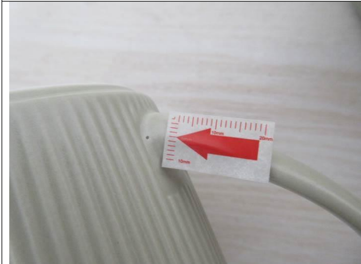
Item HTK757P: Pin hole-minor
