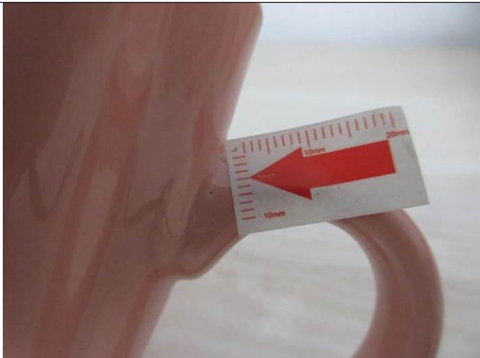
Item HTK910P:Pin hole-minor
