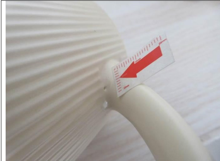
Item HTK757B: Pin hole-minor
