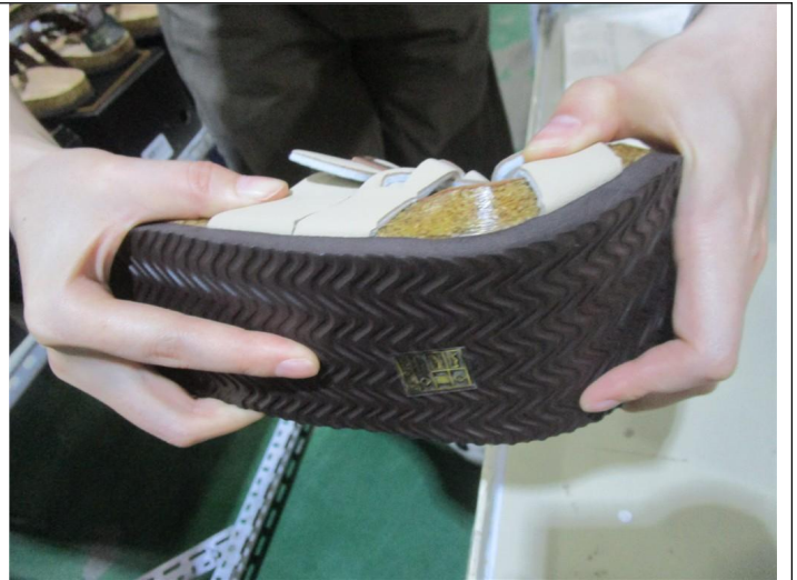
Sole bending test
