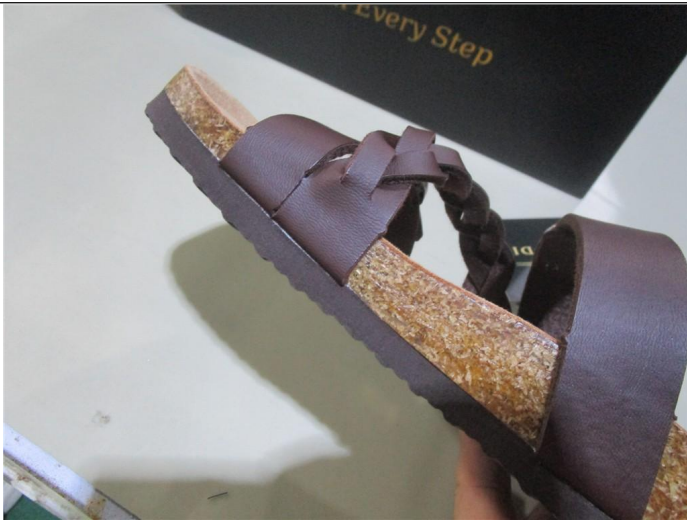
Sole bending test
