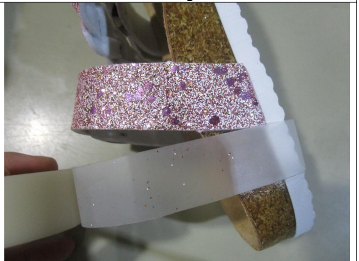
Silk Screen coating Adhesive Test
