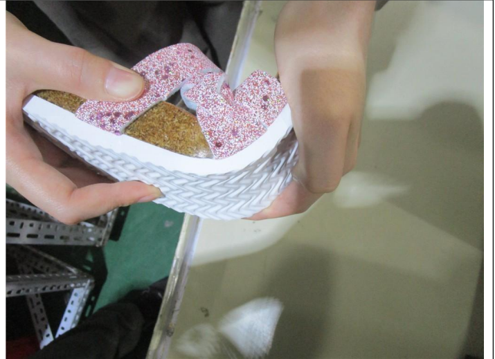
Sole bending test
