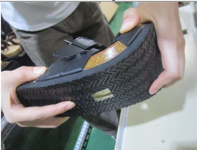
Sole bending test
