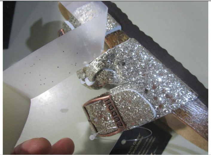
Silk Screen coating Adhesive Test
