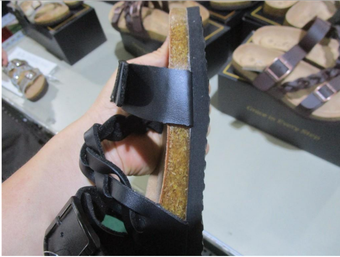
Sole bending test
