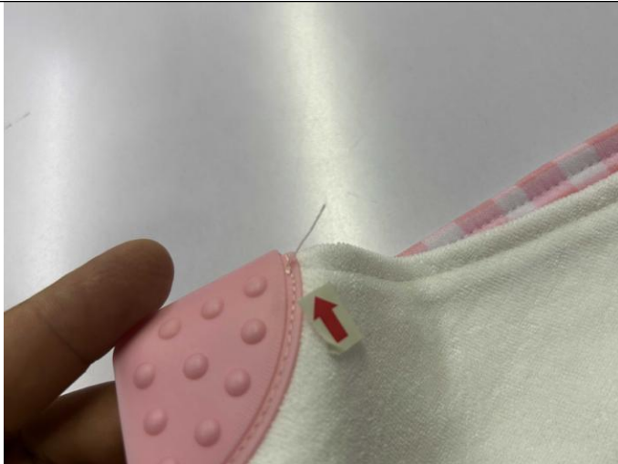
Untrimmed thread end-min
