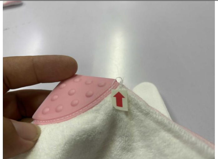
Untrimmed thread end-min
