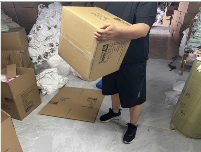
Drop test of packaging box
