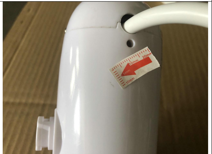
Dirty mark on unit-Minor
