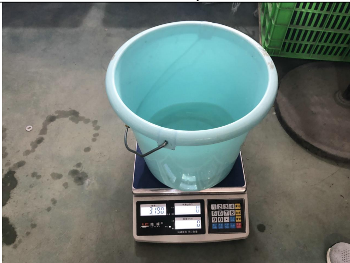
Water flow inspection
