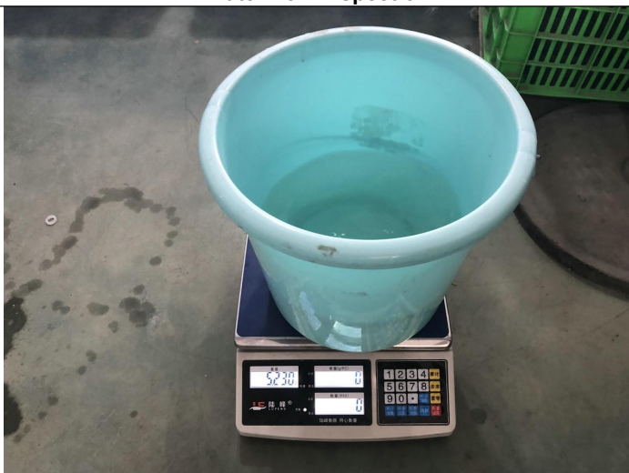
Water flow inspection
