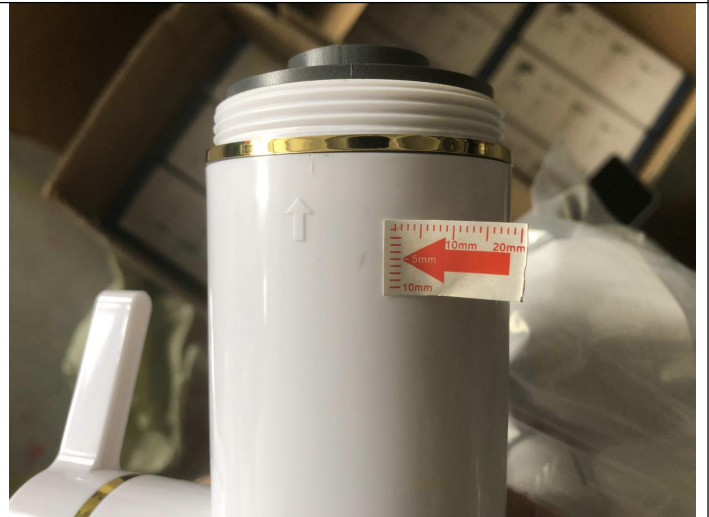
Scratch mark on unit-Minor
