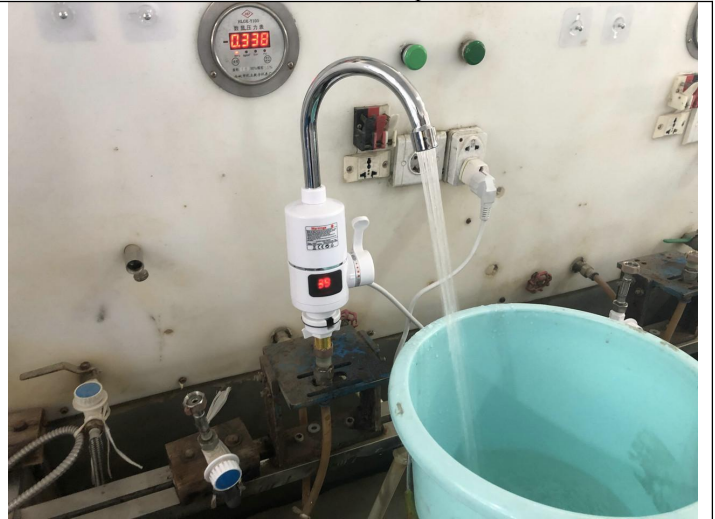
Water flow inspection
