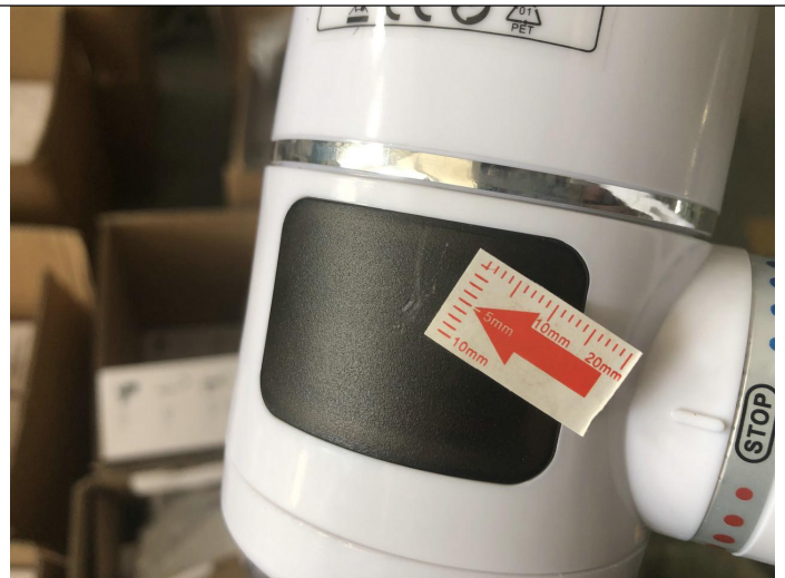
Scratch mark on unit-Minor
