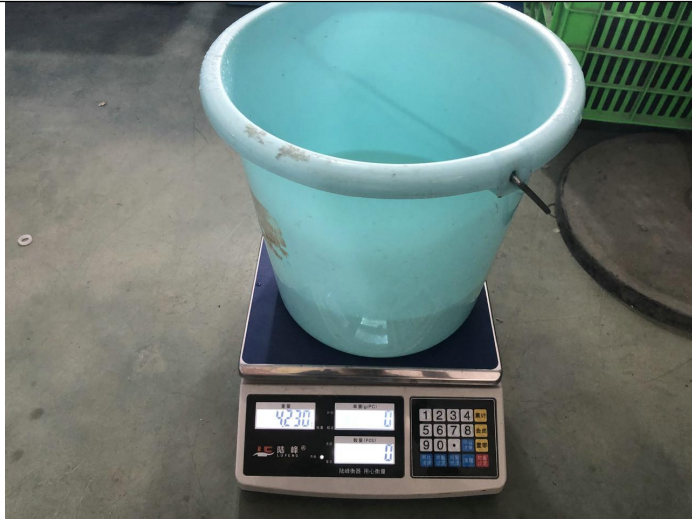
Water flow inspection
