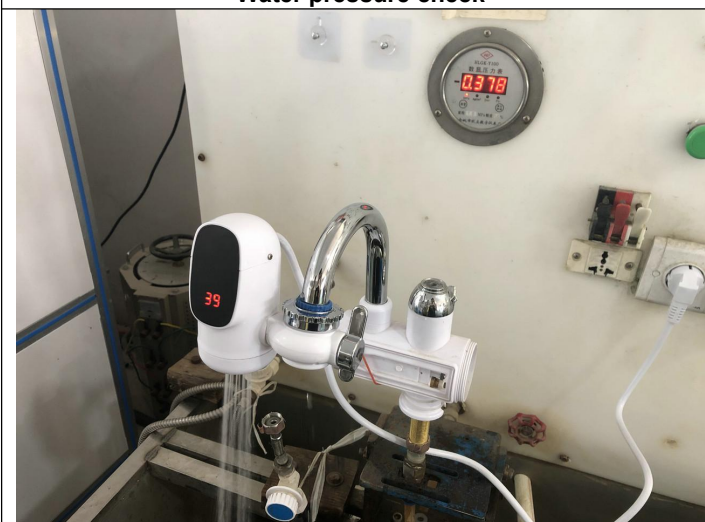
Water pressure check
