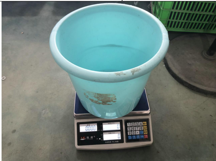
Water flow inspection
