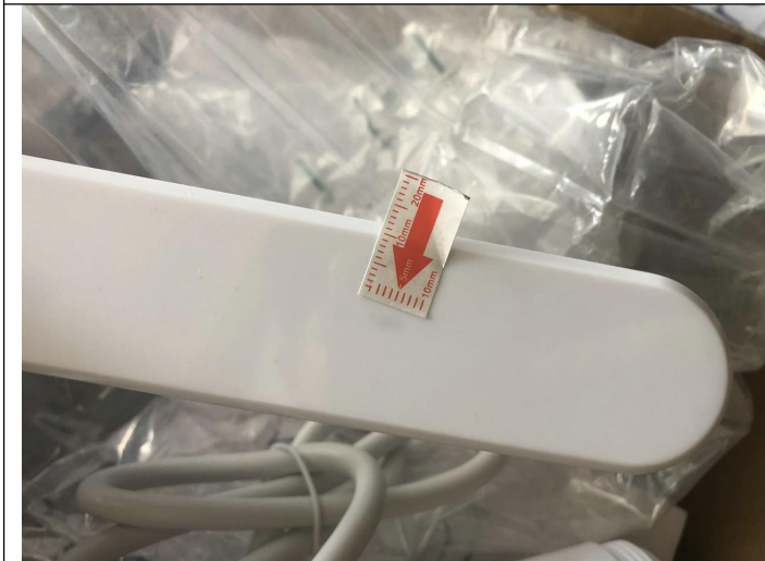
Impurity mark in unit-Minor
