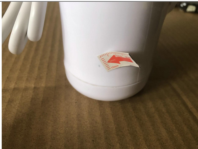
Dirty mark on unit-Minor
