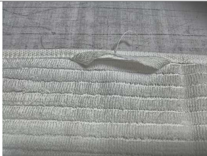
RX25110-Uncut thread ends-Minor
