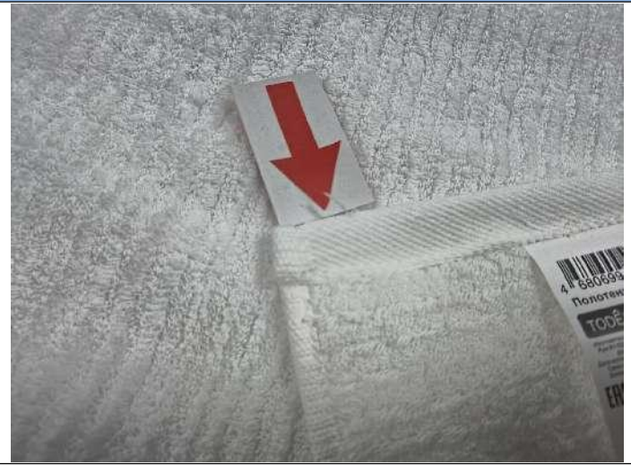
RX25110-Uncut thread ends-Minor
