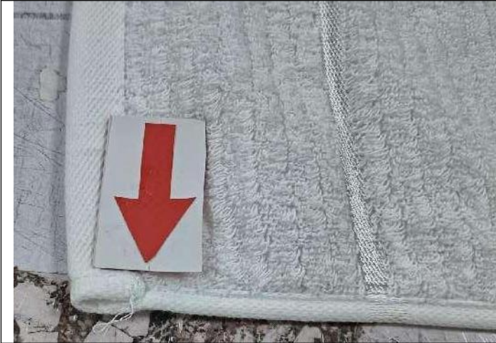
RX25102-Uncut thread ends-Minor
