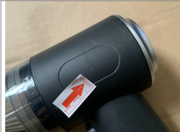
Dirty mark on unit-Minor
