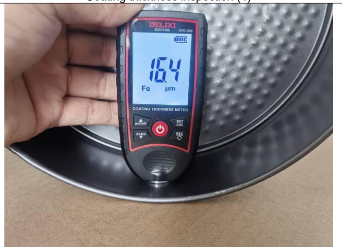
Coating thickness inspection (6)
