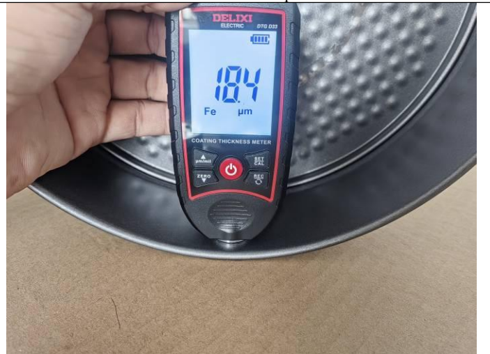
Coating thickness inspection (2)
