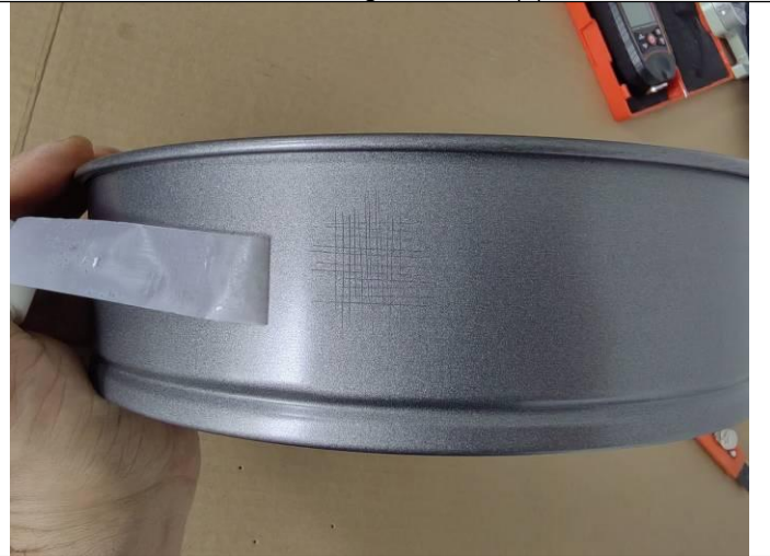
Coating Adhered Test (2)
