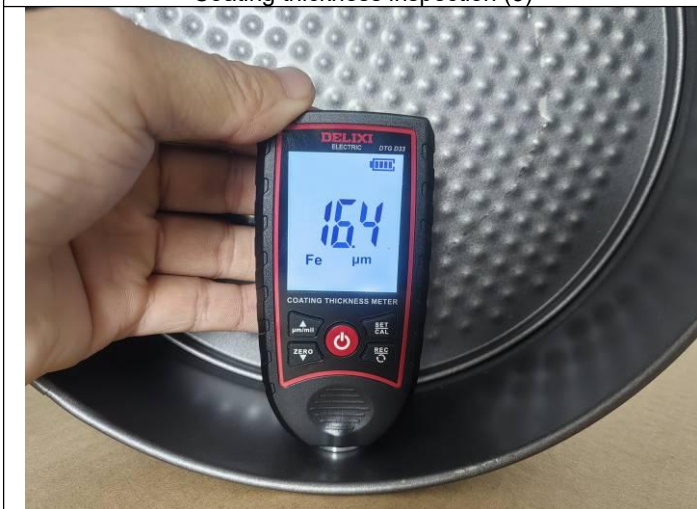
Coating thickness inspection (5)
