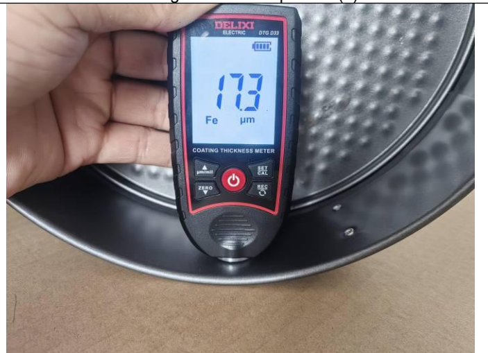
Coating thickness inspection (4)
