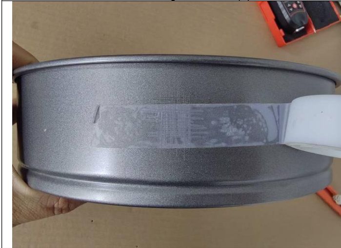
Coating Adhered Test (1)
