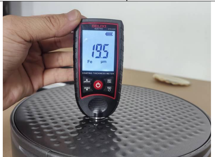
Coating thickness inspection (8)
