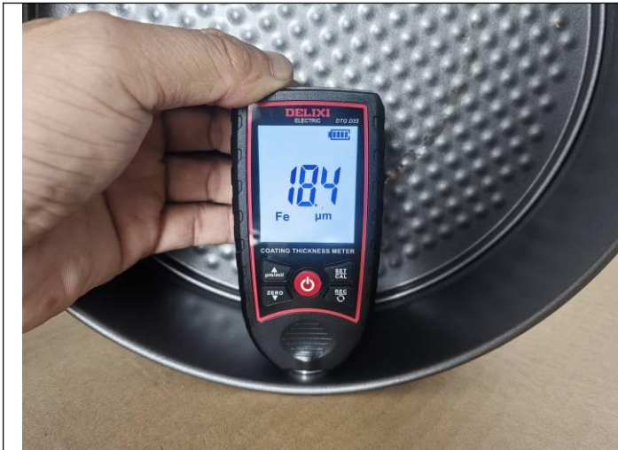
Coating thickness inspection (1)
