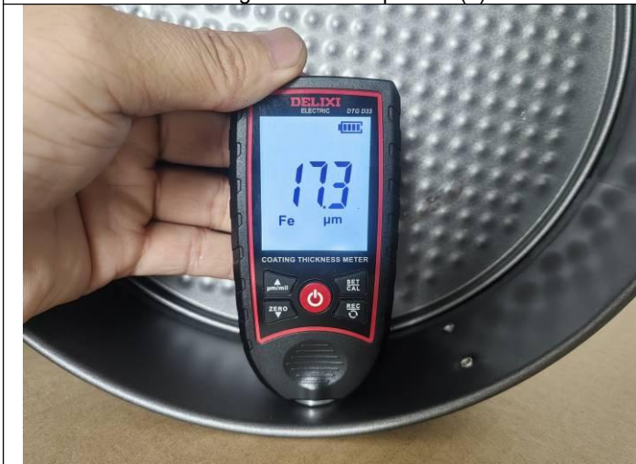
Coating thickness inspection (3)
