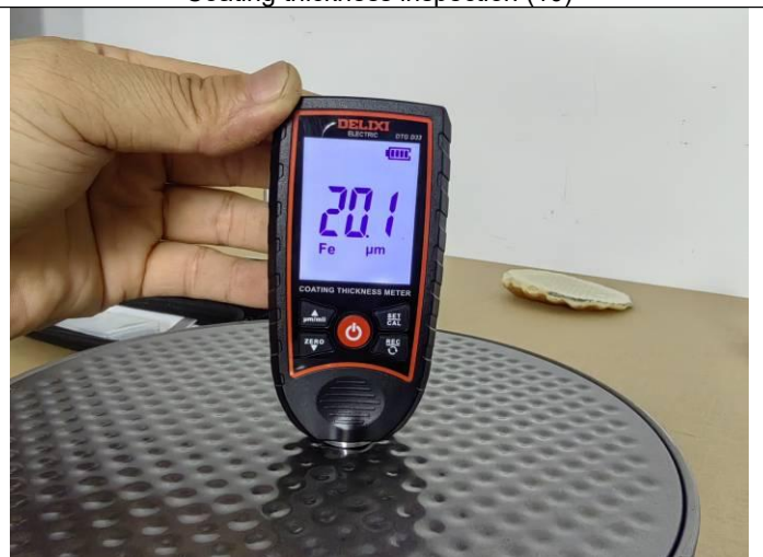
Coating thickness inspection (12)
