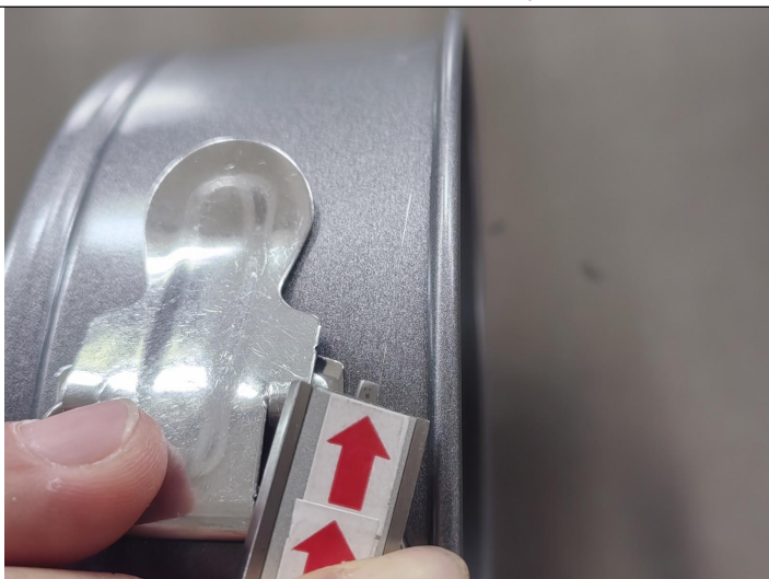
TR-TD-004 Product surface scratches -Minor
