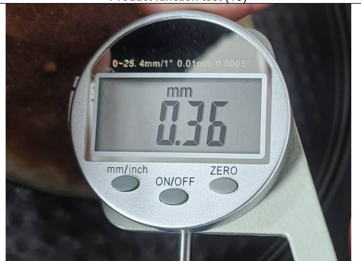
Product thickness inspection (2)
