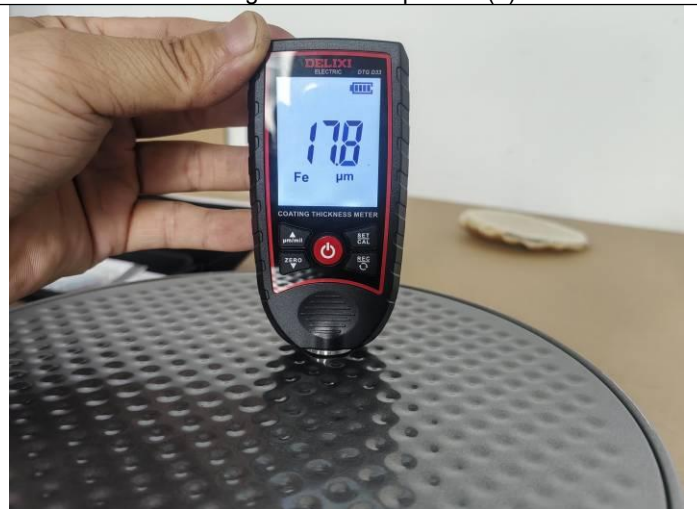
Coating thickness inspection (10)
