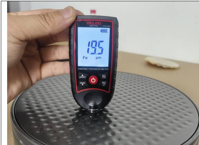
Coating thickness inspection (7)
