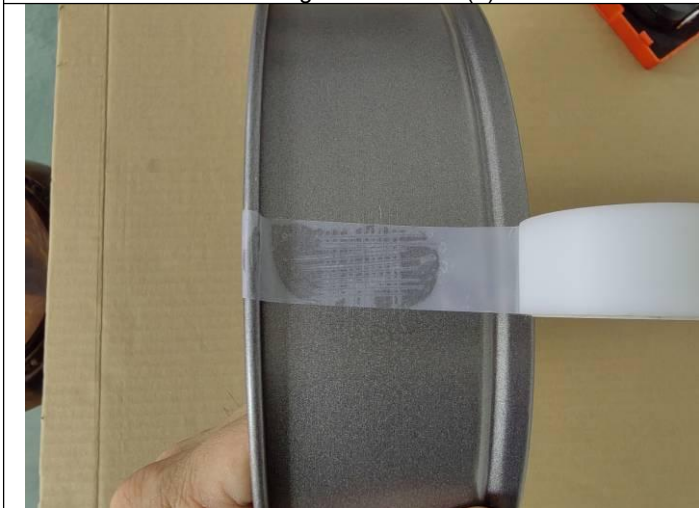
Coating Adhered Test (3)
