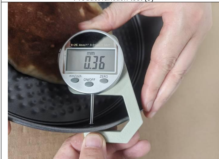
Product thickness inspection (1)
