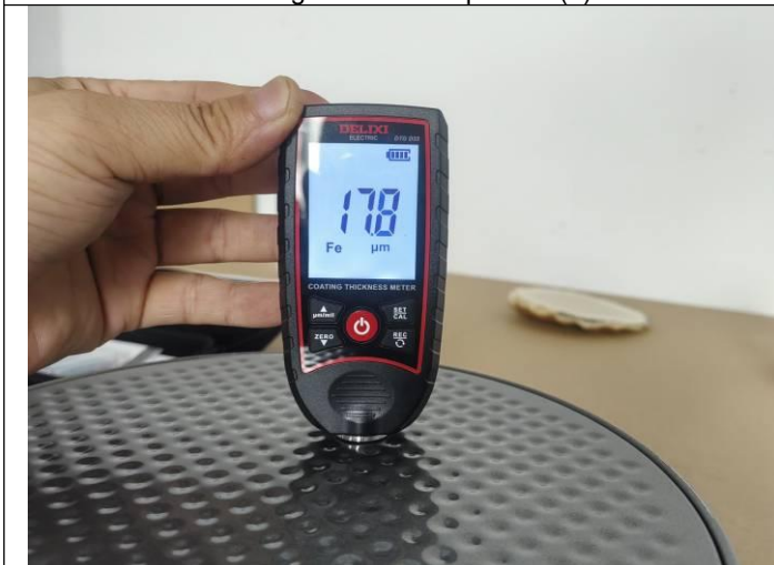
Coating thickness inspection (9)
