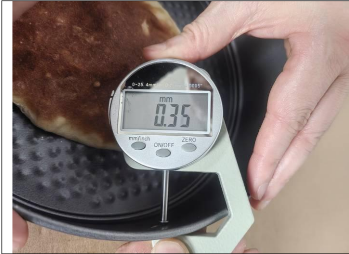
Product thickness inspection (3)
