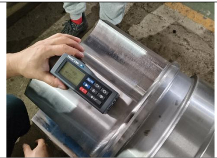
Pic.171 Surface Roughness Inspection
