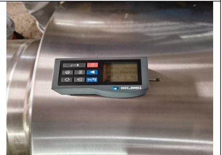
Pic.183 Surface Roughness Inspection
