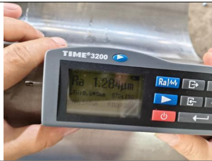
Pic.170 Surface Roughness Inspection
