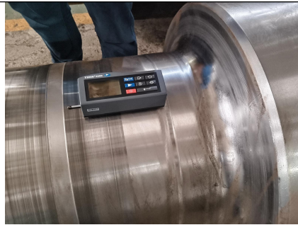
Pic.179 Surface Roughness Inspection
