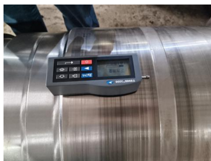
Pic.173 Surface Roughness Inspection
