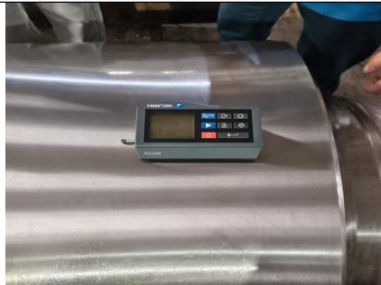
Pic.181 Surface Roughness Inspection
