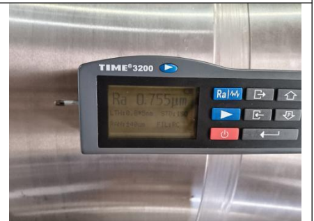
Pic.186 Surface Roughness Inspection
