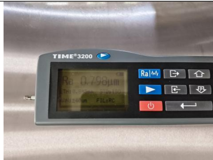
Pic.182 Surface Roughness Inspection
