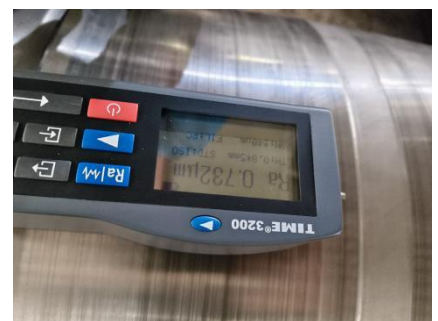
Pic.174 Surface Roughness Inspection
