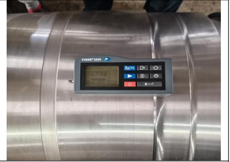
Pic.177 Surface Roughness Inspection
