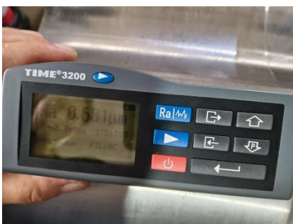
Pic.172 Surface Roughness Inspection
