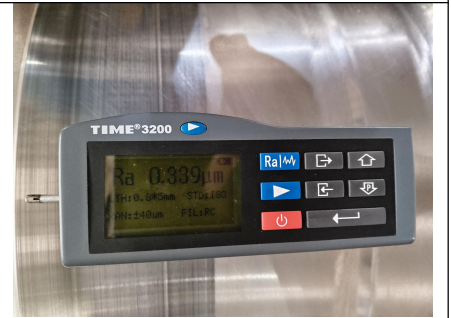
Pic.180 Surface Roughness Inspection
