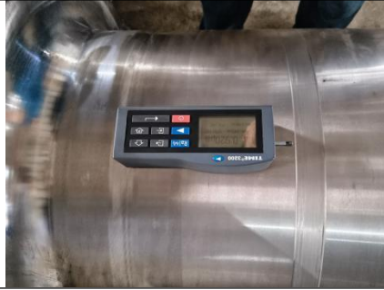
Pic.175 Surface Roughness Inspection
