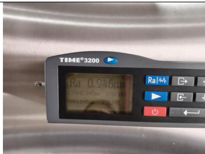
Pic.184 Surface Roughness Inspection
