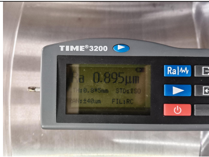
Pic.178 Surface Roughness Inspection
