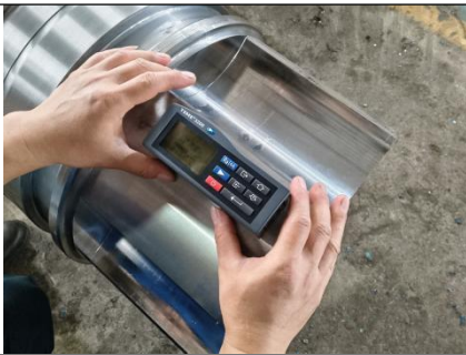
Pic.169 Surface Roughness Inspection
