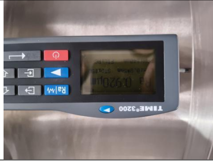
Pic.176 Surface Roughness Inspection
