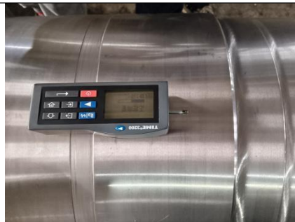
Pic.185 Surface Roughness Inspection
