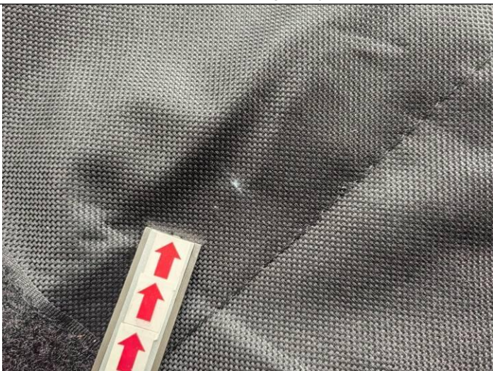
Dirty mark at surface-Minor
