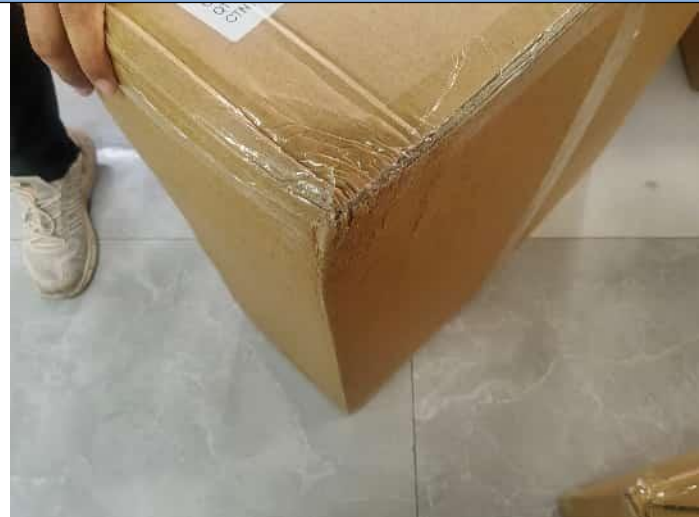
Drop test of packaging box
