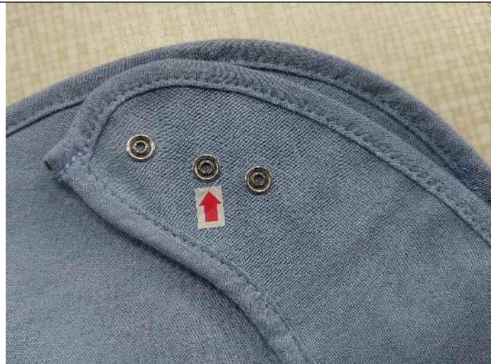
9.The sewing crease issue on the blue Bib (30×60 cm) accounts for 10%.
