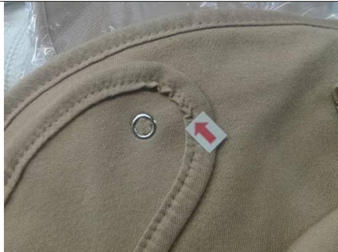
8.The issue of inaccurate button placement on the blue Bib (30×60 cm) accounts for 12%.
