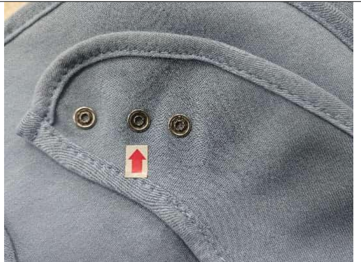
8.The issue of inaccurate button placement on the blue Bib (30×60 cm) accounts for 12%.
