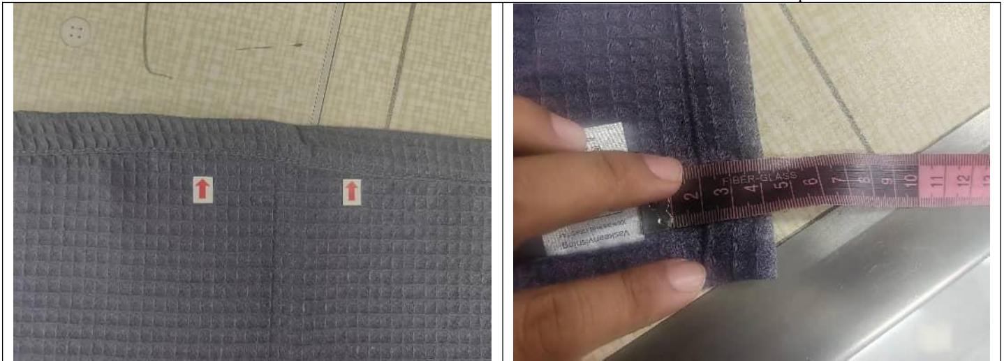
The edge lines are not aligned-Maj
